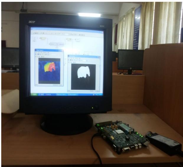
Fig. 15 Hardware co-simulation for segmentation using XSG
