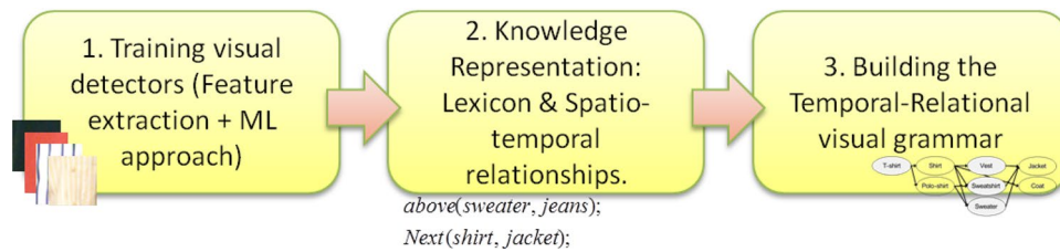
Fig. 2 Schema of the training phase of our method. It consists of three main blocks: In the first stage it extracts visual features and trains the garment detectors with a machine learning approach. In
