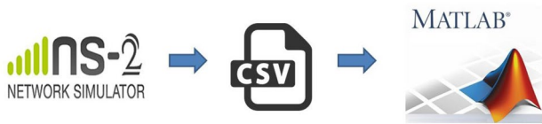
Fig. 4 The simulation methodology; generating initial population using NS-2 and then it is fed to Matlab to execute the genetic algorithm and produce the best possible paths
