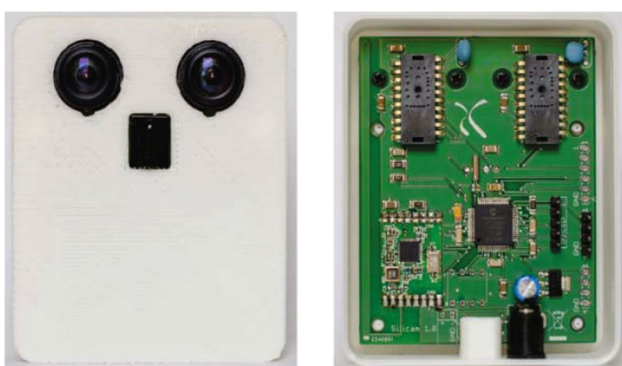
Fig. 1 The camera consists of stereo pair of image sensors controlled by a digital signal controller. Each image sensor delivers an image with a resolution of 30 \times 30 pixels
