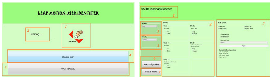
Fig. 4 a Identification interface. The figure is tagged with (1) sweet spot indications—the arrows indicate the direction in which the user has to move the hand; (2) recognition feedback; (3) link to the training interface and (4) link to reset the workflow. b Interface for space customization. The figure is tagged with different numbers: (1) The
