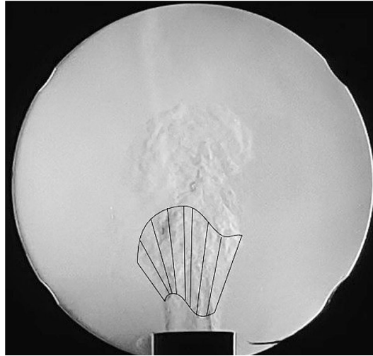
Fig. 6 “S” wave formed in S30-1-D in sinusoidal orifice geometry
