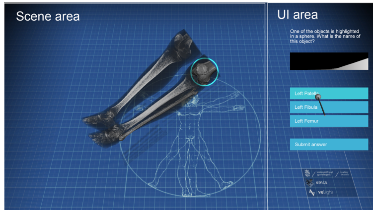
Fig. 4 The interface: the right part of the screen is the UI Area, the left part is the Scene Area. In this particular task, the user has to select the highlighted object in the volume rendering. The UI Area contains the question, the transfer function of the volume, the multiple choices and a submit button
