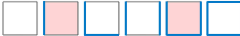
Fig. 17 Locating degenerate points (Bi et al. 2010a). Each square contains four tensor samples on the four vertices. The edge in blue is a degenerate pair. The square is shaded in red if it contains a degenerate point
