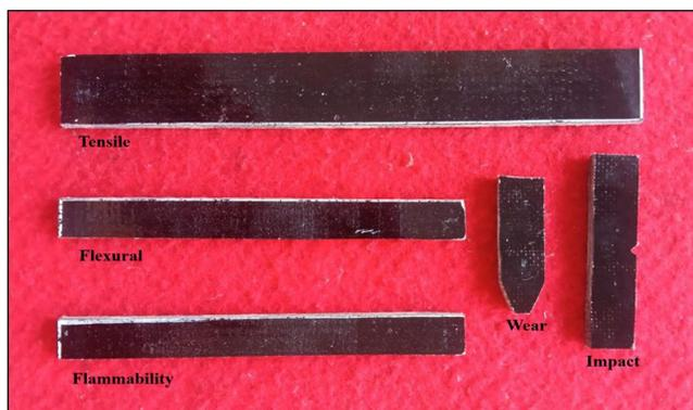
**Fig. 5** ASTM standard testing specimen for lignin and abaca polyester composite
