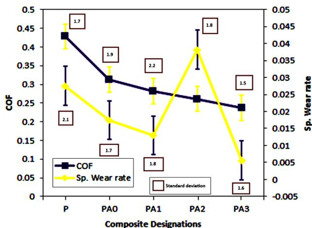
Fig. 7 Wear properties for various composites
