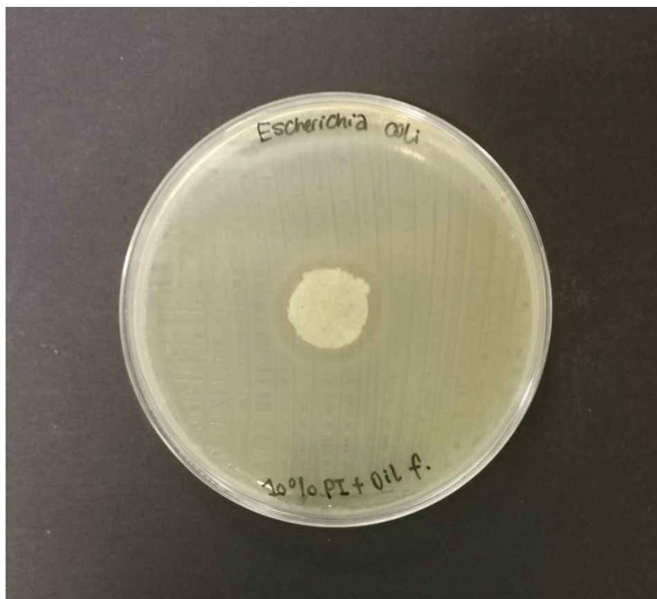
Fig. 3 The images of disc diffusion assay of films containing 10% protein isolate (PI) and pepper oil (10PI + PO) against Escherichia coli
