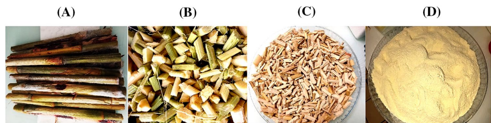
Fig. 1 Biomass pretreatment operations: cut stalk (A), Marrow (B), whole deleafed stalk cut up and dried (C) and ground stalk (D)
