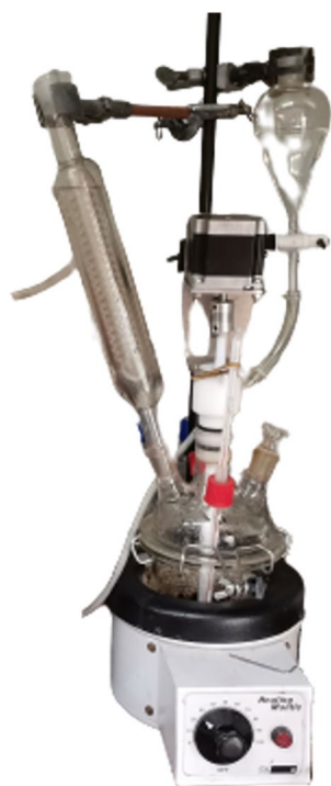
Fig. 1 Experimental setup used for the one-pot phenolation and LPF synthesis
