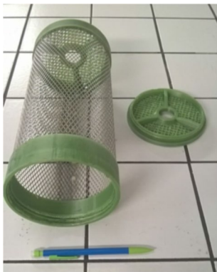
Fig. 2 Picture of one capsule used to feed the micro-scale AD prototype along periods 2 and 3
