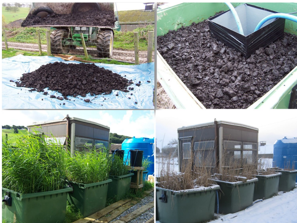
Fig. 5 Field study of AIS-based CW for animal farm wastewater treatment
