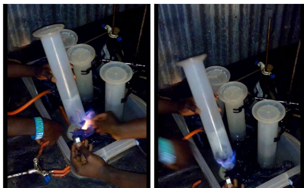
Fig. 7 Flammability test on biogas produced from the experiments
