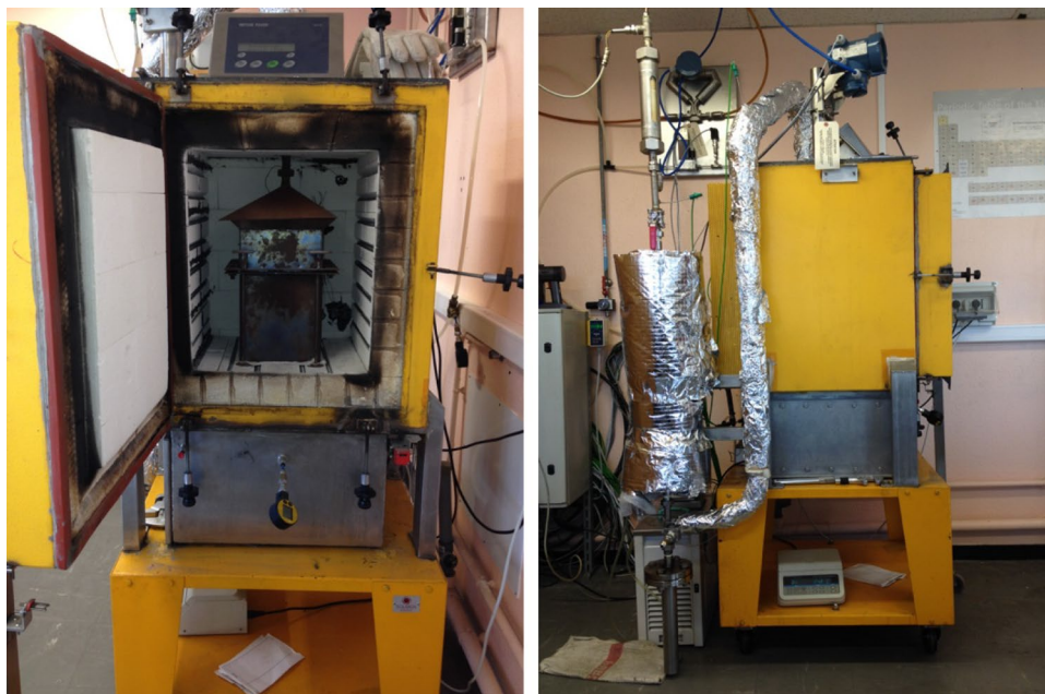
Fig. 14 High capacity thermobalance at LaTEP ( left front view, right side view )
