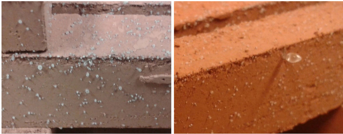
Fig. 6 Entrapped gas pockets at the surface of bricks containing 15 % of glass wastes (GW)
