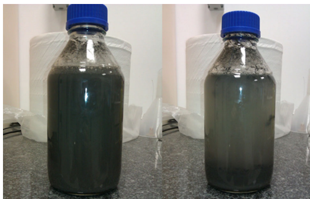
Fig. 7 Images illustrating delamination of fertilizer suspension based on ashes
