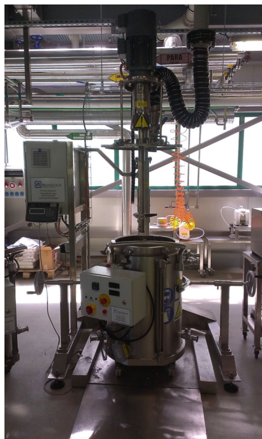
Fig. 2 The experimental pilot plant for liquid fertilizer production
