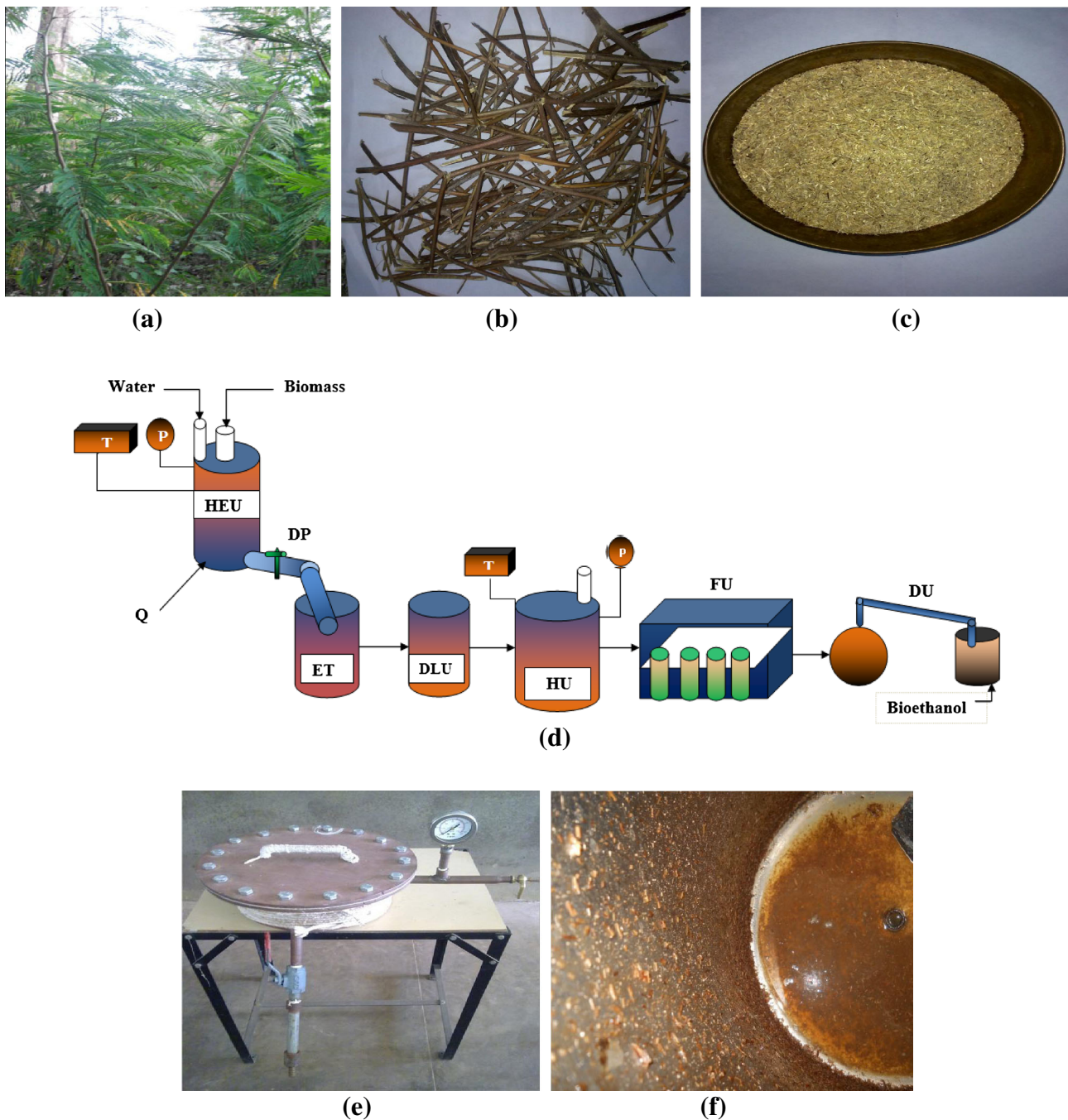
Fig. 1 a Calliandra calothyrsus shrub. b Stem of Calliandra calothyrsus . c Raw material. d Line diagram of bioethanol production, T temperature sensor, P pressure sensor, HEU hydrothermal explosion unit, ET explosion tank, DLU delignification unit, HU
