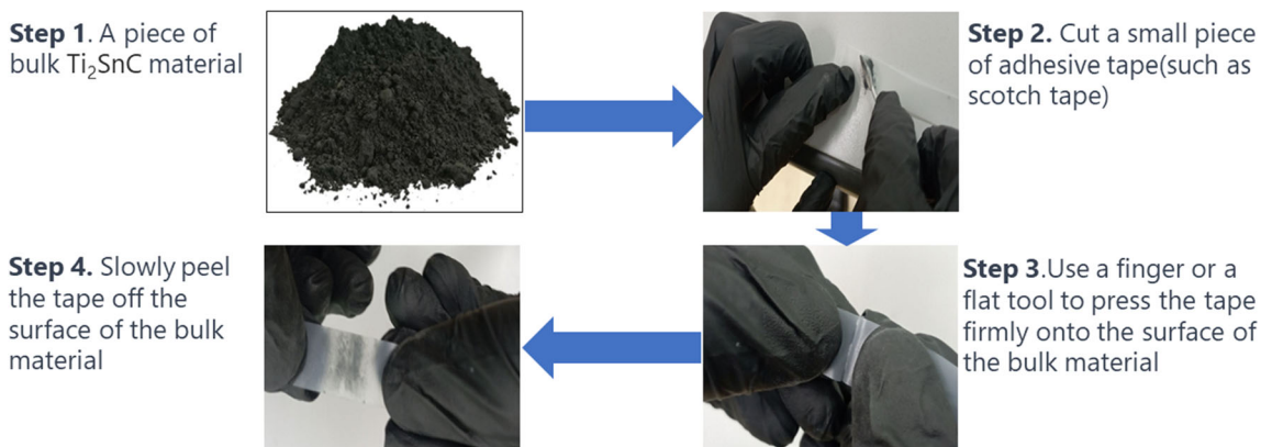
Fig. 1 The process of mechanical exfoliation method
