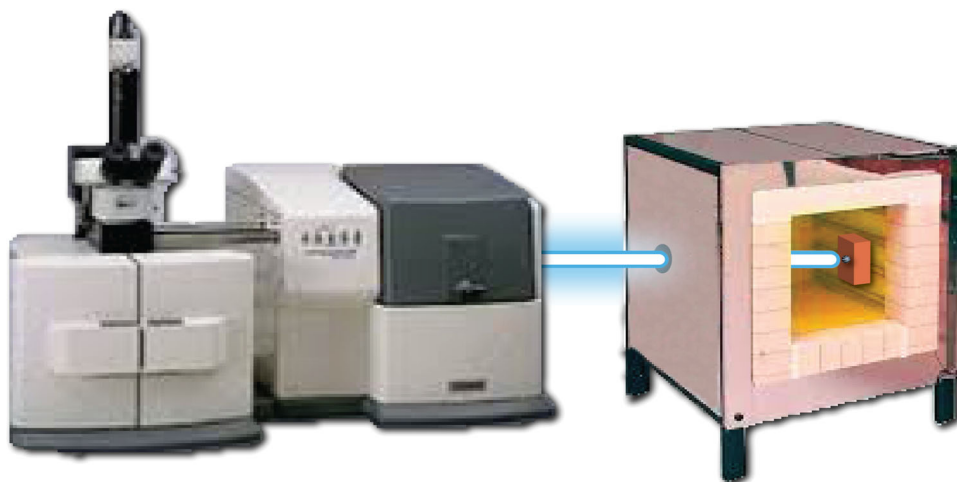
Fig. 2 How to irradiate a laser beam on the TiO 2 anatase tablet in a furnace by increasing the temperature
