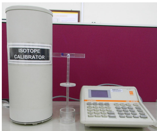
Fig. 4 Radionuclide calibrator with source holder for placing the vial, electrometer and readout console in BARC
