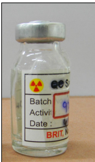
Fig. 6 Sealed injection glass vial with ^{131}\text{I} radioactive solution calibrated at BARC and then despatched to NMC
