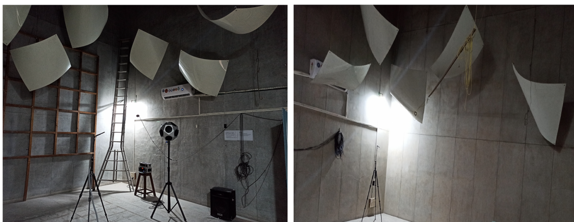
Fig. 2 Pictorial view of reverberation chambers used for airborne sound insulation measurements and diffusers installed for ensuring sound diffusivity at CSIR-National Physical Laboratory, New Delhi
