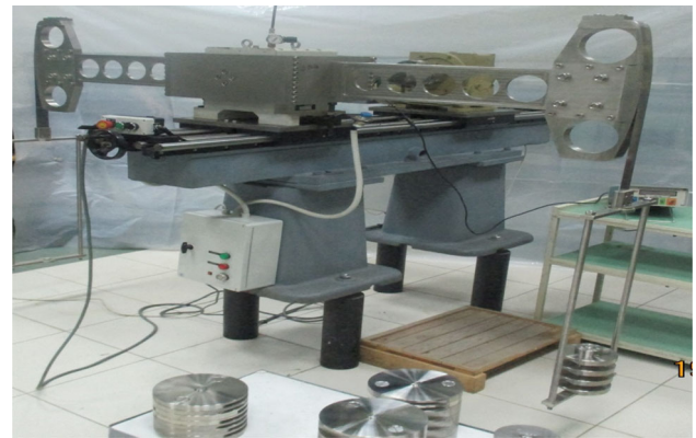
Fig. 11 NIS 1 kN-m primary torque standard machine
