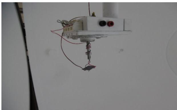
Fig. 10 LED on Substrate sample inside the Light output testing sphere
