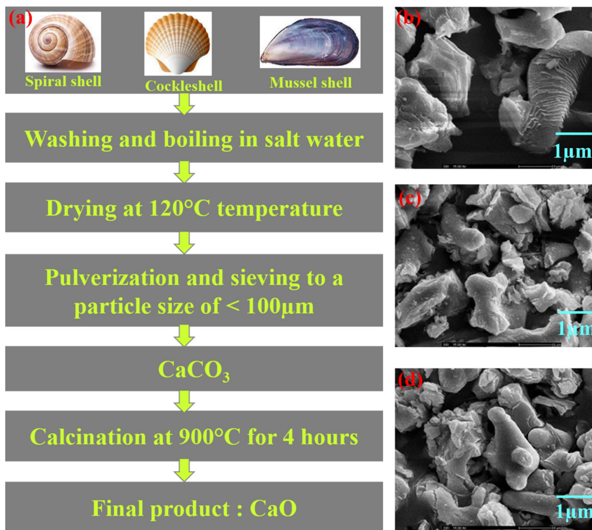
Fig. 4 (a) Flowchart for the obtaining of calcium carbonate and calcium oxide from sea shells. [55] SEM image of (b) mussel shell (c) cockle shell (d) scallop shell calcinated at 1000 degree celsius. [61]
