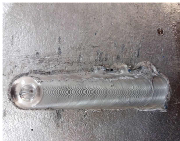
Fig. 1 A typical friction stir processed Al–20Si alloy plate
