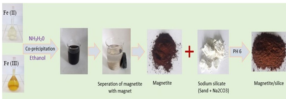
Fig. 1 Synthesis of \text{Fe}_3\text{O}_4 and \text{Fe}_3\text{O}_4 @\text{SiO}_2
