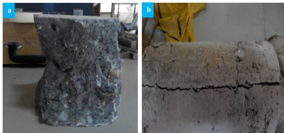
Fig. 6 Failure of SCC (a) Compression and (b) Tensile [44]
