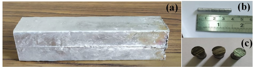
Fig. 2 a Cast product of Al-Ni-SiC composite, b wear sample before test c wear sample after test
