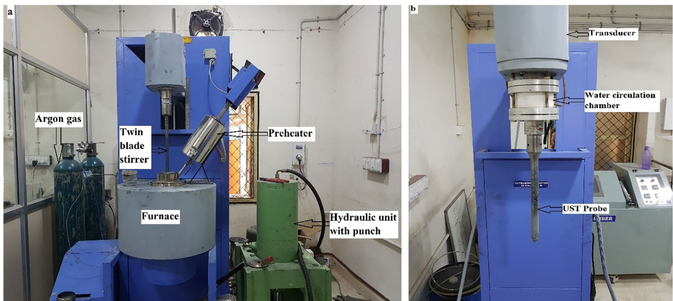
Fig. 1 (a) Magnesium Squeeze casting setup and (b) Titanium Ultrasonication probe
