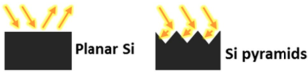
Fig. 5 Light-matter interaction on planar Si and Si pyramids
