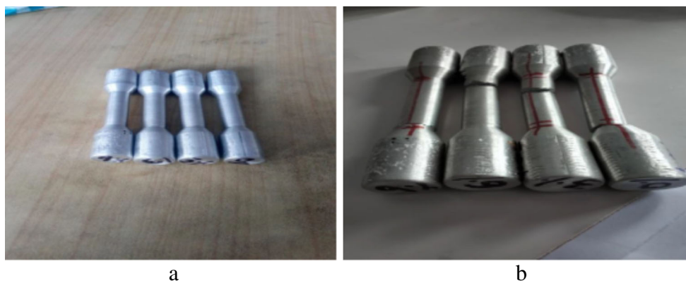
Fig. 2 Tensile test specimen before testing (a) and after testing (b)
