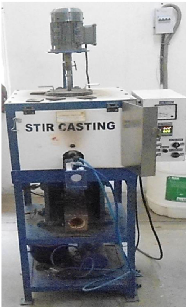
Fig. 1 Stir casting set up for HMMCs
