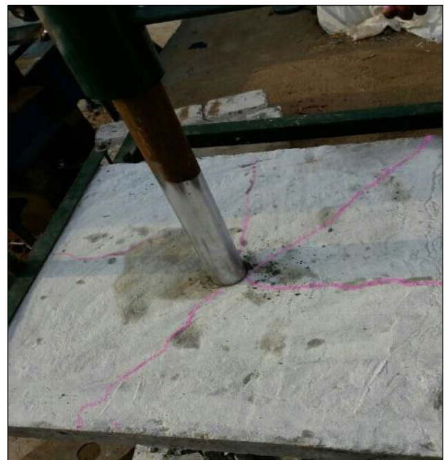
Fig. 3 Slab under impact load test
