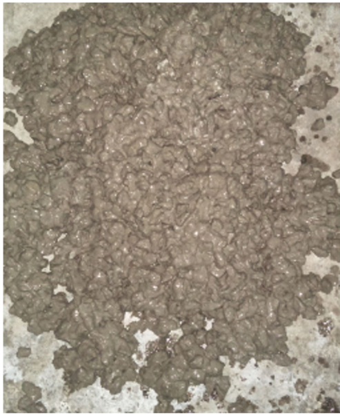
Fig. 4 Geopolymer concrete in fresh mix condition
