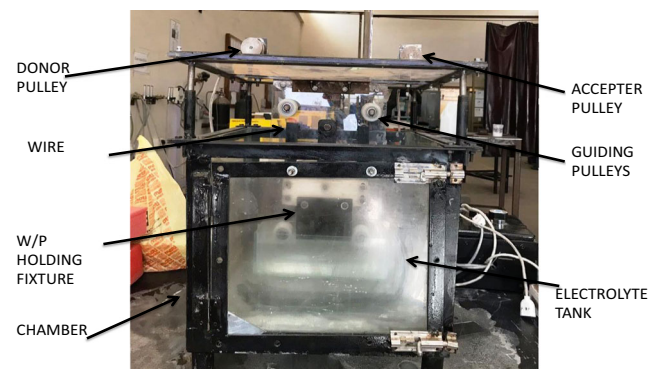
Fig. 2 In-House developed TW-ECDM setup
