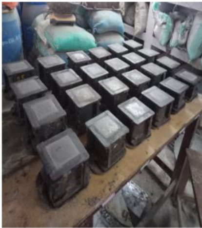
Fig. 14 Casting of HSC specimens
