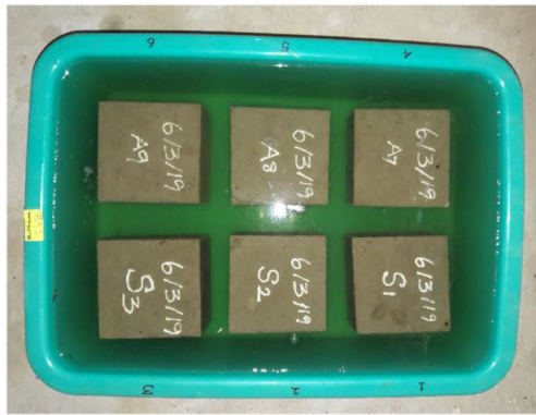
Fig. 16 Sulphate attack test
