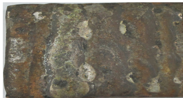
Fig. 1 Hardfacing coating after welding
