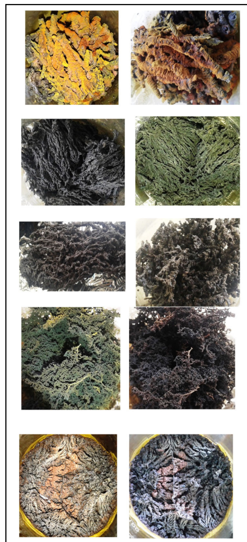
Fig. 4 a-e: Image of as prepared ferrites showing the fractal patterns: a Cd-ferrite, b Cr-ferrite, c Cu-ferrite, d Li-ferrite and e Mg-ferrite
