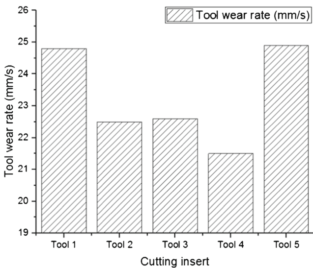
Fig. 10 Effects of various types of microgroove geometry on tool wear rate
