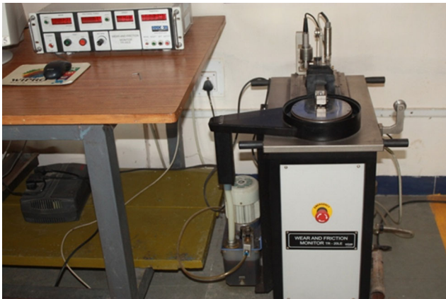
Fig. 2 Dry sliding wear test rig
