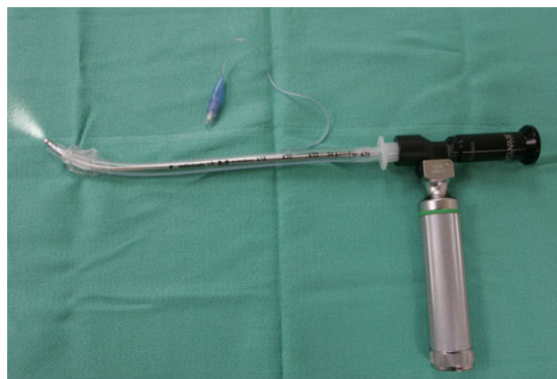
Fig. 1 The Levitan FPS (first pass success) scope (LFS) is a short malleable semi-rigid fiberoptic stylet developed by Richard Levitan and manufactured by Clarus Medical (Minneapolis, MN, USA). Image courtesy of Dr. Orlando Hung
