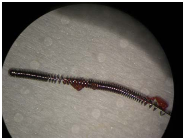
Fig. 1 Distal portion of the Stimucath ® stimulating catheter following surgical removal after an otherwise functionally successful interscalene block. Note the partial uncoiling and catheter tip elongation, and absence of knotting
