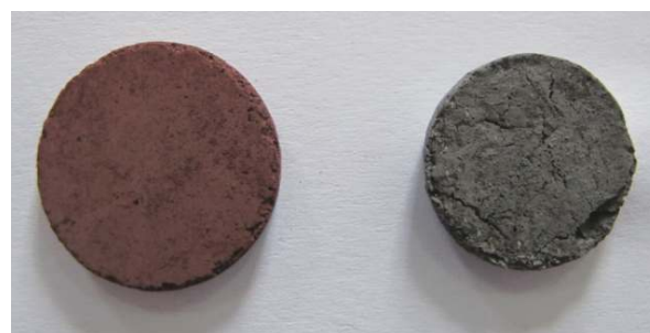
Fig. 8. Digital photos of mixed NiO and Fe 2 O 3 pellets before (left) and after (right) electrolysis at 750°C with a cell voltage of 1.9 V in a Na 2 CO 3 –K 2 CO 3 eutectic melt for 11 h.
