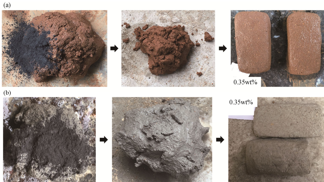
Fig. 1. Sequential images for the preparation of (a) graphene-reinforced burnt red soil brick and (b) graphene-reinforced fly ash brick nanocomposite (both containing 0.35wt% graphene).
