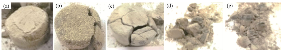
Fig. 11. Failure modes and destruction degree of Group 70-6-90: (a) No. 70-6-90-1; (b) No. 70-6-90-2; (c) No. 70-6-90-3; (d) No. 70-6-90-4; (e) No. 70-6-90-5.
