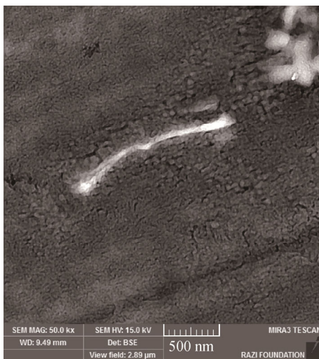
Fig. 12. Microscopic image of the fusion zone of the sample subjected to the second heat-treatment cycle.
