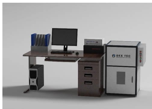
Fig. 3. Ultrasonic fatigue testing machine used in this work.
