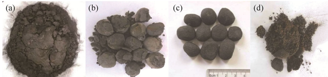
Fig. 3. Photographs of the pellets reduced at different temperatures: (a) 900°C; (b) 1000°C; (c) 1150°C; (d) 1200°C.
